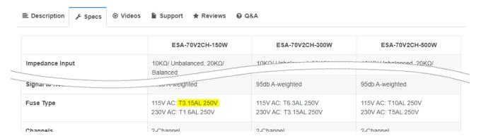
Take that 3.15 amps and multiply it by the standard North American power grid rating of 120 volts. 3.15A × 120V = 378W.
