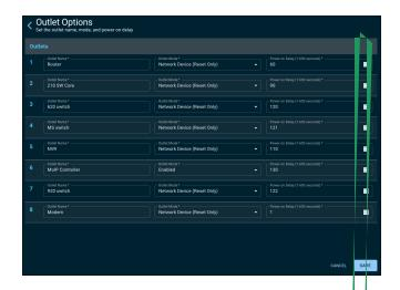
**Tip:** Configure the **Outlet Mode** to **Network Device (Reset Only)** for all network devices to avoid outages caused by devices accidentally being powered off.
