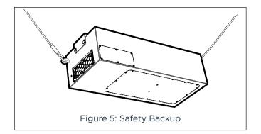
5. Recommended: for safety backup, connect eyebolts and rigging (not included) to the builtin M10 flypoints on both ends of the cabinet. Consult a structural engineer on every installation to ensure the appropriate hardware and rigging are implemented in accordance to local code and regulations (see Figure 5).
