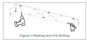
Secure the bracket to the installation surface. Use high-quality, graded lag bolts or similar fasteners rated for > 150 lbs (180kg) each of shear working load. M10 or 3/8" bolts are recommended. To prevent excessive vibration transference, use a damping material (such as mass-loaded vinyl, neoprene foam, rubber sheets, etc.) between the bracket and installation surface (see Figure 2).
