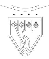
Connect the positive (+) and negative (-) speaker cable to the left + and right - screw terminals. Use the right + - terminals to link to another speaker.
