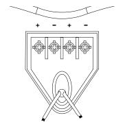
③ Run the speaker cable through the tube positioned at the rear of the cabinet to the terminal at the front baffle.
