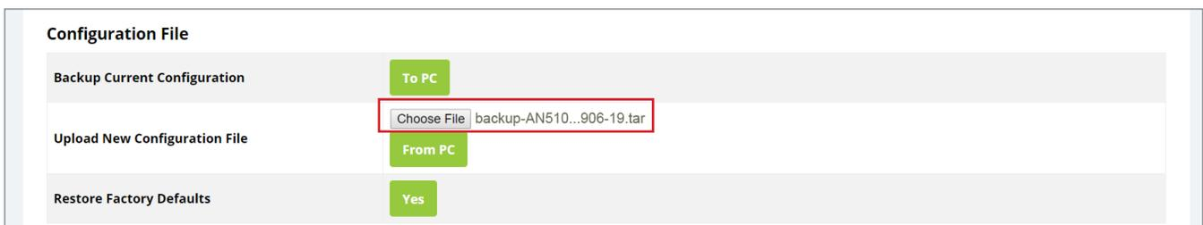
3. Click the From PC button to upload the configuration file. Wait while the Rebooting screen opens and loads the selected configuration. When the upload is finished, the Authentication Required (Log In) window will open.
